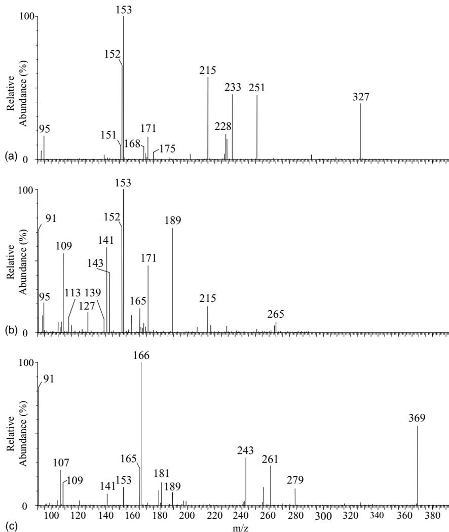
Fig. 5. CID spectra of (a) triphenyl phosphate  $m/z$  327 (scan range  $m/z$  90–350); (b) diphenyl methyl phosphate  $m/z$  265 (scan range  $m/z$  90–290); and (c) tritolyl phosphate  $m/z$  369 (scan range  $m/z$  90–400). The collision energy was set to 25 eV.
