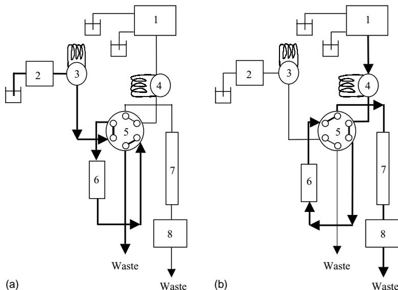
Fig. 2. Schematic diagram of the on-line SPE/HPLC system used for the extraction of organophosphorus triesters from human blood plasma. Parts (a) and (b) illustrate the loading mode and the analysis mode, respectively. (1) HPLC pump; (2) auxiliary pump; (3, 4) injection valves; (5) column switch valve; (6) RAM column; (7) HPLC column; and (8) detector.
