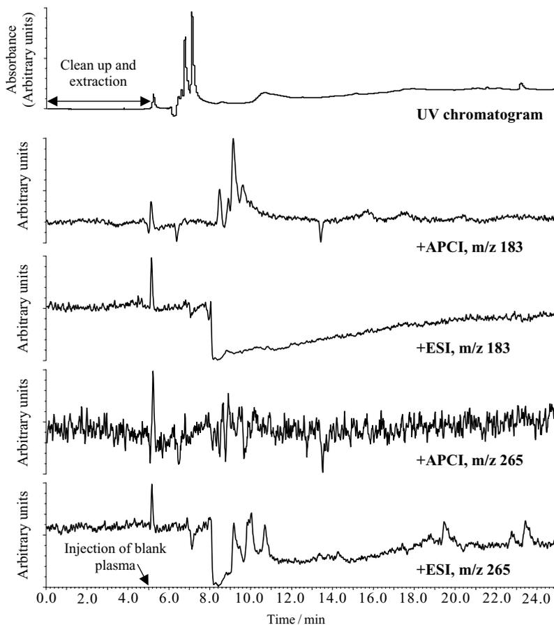
Fig. 3. UV and extracted ion chromatograms of post-column infusion of triethyl phosphate ( $m/z$  183) and diphenyl methyl phosphate ( $m/z$  265) into extract of blank plasma. The compounds were ionized using +APCI and +ESI.
