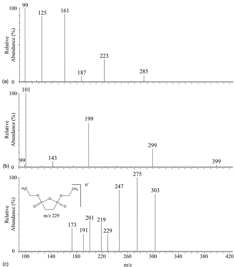
Fig. 4. CID spectra of (a) tris(2-chloroethyl) phosphate  $m/z$  285 (scan range  $m/z$  90–310); (b) tris(2-butoxyethyl) phosphate  $m/z$  399 (scan range  $m/z$  90–425); and (c) tetraethyl ethylenediphosphonate  $m/z$  303 (scan range  $m/z$  90–330). The collision energy was set to 16 eV.
